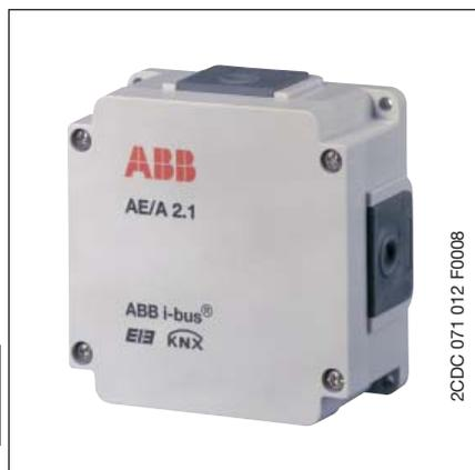
Analogue Input AE/A 2.1 is used to record analogue data. Two conventional sensors can be connected to AE/A 2.1. The connection to the bus is established using a pluggable screw terminal. The device is ready for operation after connecting the bus voltage. No additional auxiliary voltage is required. Analogue Input AE/A 1.2 is parameterised and programmed using the ETS (ETS2 V1.3a).
