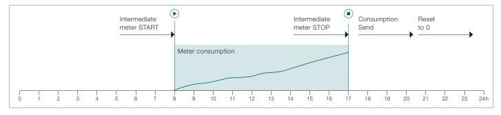
The intermediate meters of the individual energy actuators are synchronized once a day by a bus telegram. The meter reading is sent cyclically on the bus. Energy consumption curves can be represented in this way for all loads. This function can be applied for the comparison of energy consumption in lighting or air-conditioning of manufacturing or storage facilities at freely definable intervals (week, month, year).
