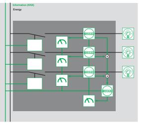
The Energy Actuator facilitates control of the connected consumer loads via the ABB i-bus<sup>®</sup> KNX. For each of the three switch channels, the individual consumption can be measured in the same way as for the Energy Module. For every channel, the proven functionality of the ABB i-bus<sup>®</sup> KNX Switch Actuators are available.
