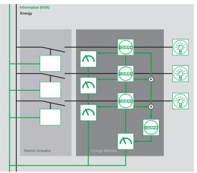
The Energy Module can record the energy consumption for the individual devices. It is used particularly when upgrading existing KNX systems and wherever energy measurement is required without switch functions. It facilitates a detailed and transparent insight into the energy consumption of a building.
