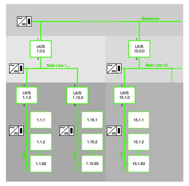
Backbone = Area line with up to 15 area couplers, physical address x.0.0
