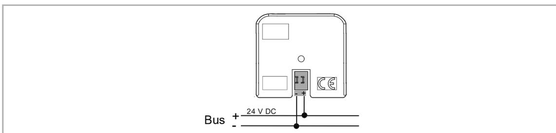
Fig. 4: Electrical connection
