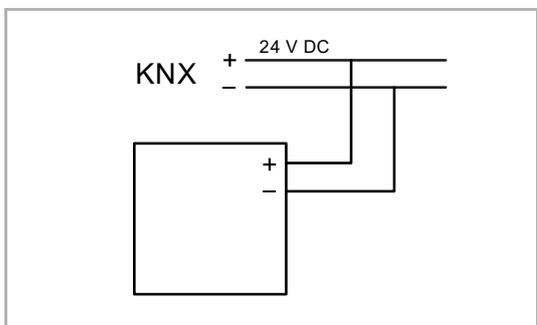
Carry out the electrical connection according to the circuit diagram.
