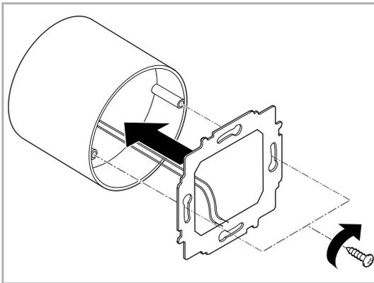
1. Screw the support ring to the flush-mounted box.
