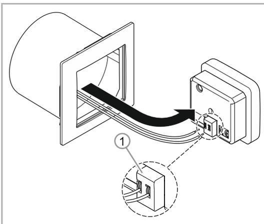
3. Connect the bus line with the bus connection terminal [1] (Chapter 6.2 "Electrical connection" on page 15).
