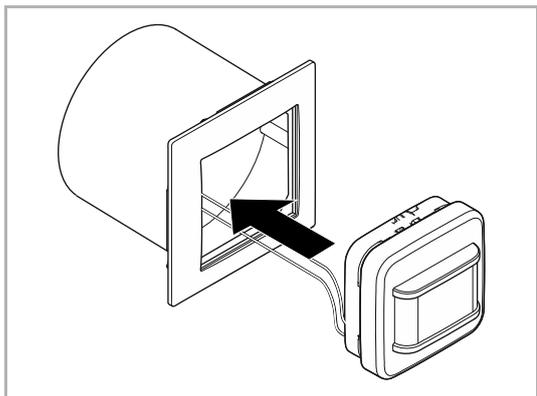
6. Snap the device into the support ring.
