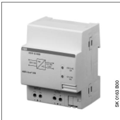
The power supply unit is a DIN rail mounted device for insertion in the distribution board. It provides a regulated output voltage of 12 VDC with a maximum output current of 1.6 A as an auxiliary supply in EIB installations or other SELV applications.
