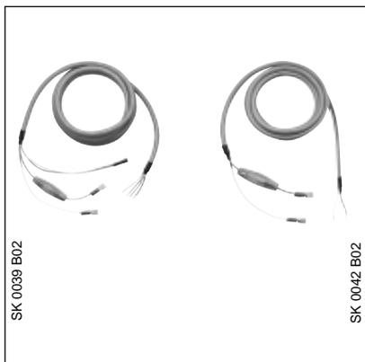
The Cable Set Basic KS/K 4.1 (for one battery) or both Cable Sets Basic KS/K 4.1 and Extension KS/K 2.1 (for two batteries in parallel) must be used for the connection of a sealed lead acid battery to the Uninterruptible EIB Power Supply SU/S 30.640.1. The Battery Module AM/S 12.1 can be wired using a standard cable.
