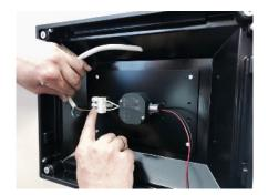
Step 5 A protective conductor is mounted on the back of the square. Connect this protective earth cable to the free PE terminal of the device connection terminal.
