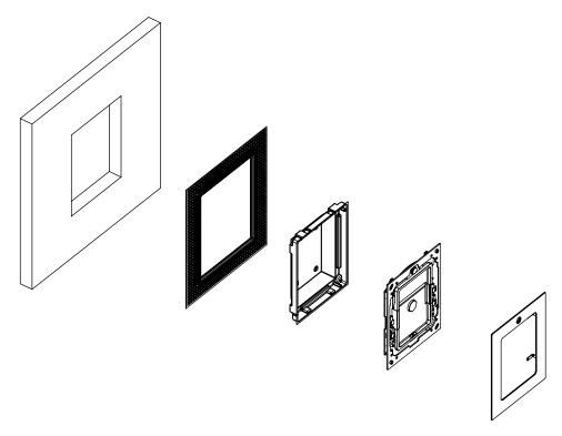
Install the flush box so deep that it rests firmly on the inner ring of the frame.
