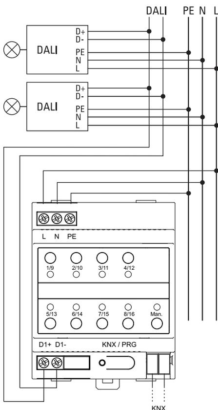
Once all connections are complete and the supply voltage has been switched on, the DALI line can be commissioned and programming carried out with the ETS.
