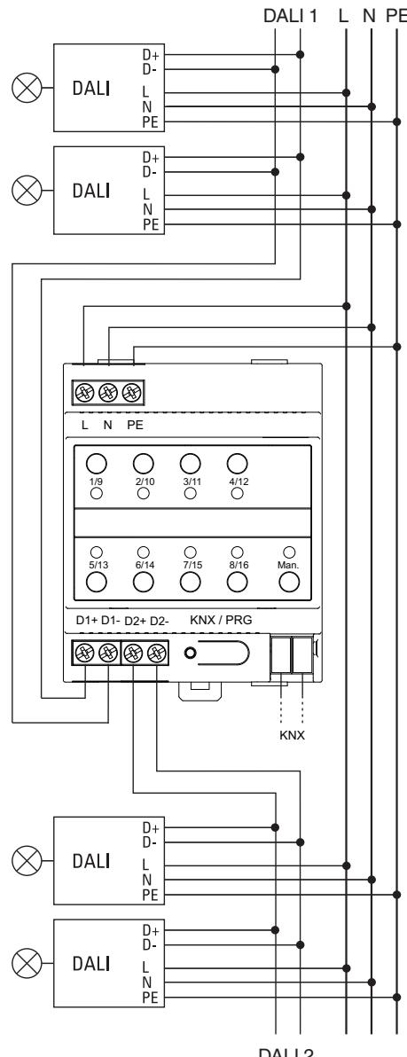
Once all connections are complete and the supply voltage has been switched on, the DALI line can be commissioned and programming carried out with the ETS.
