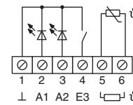
Binary outputs A1, A2: Connect LED or electronic relay to terminal strip between terminals 1 and 2...3.
