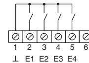
Binary inputs E1...E4: Connect window contact, make or break pushbutton to the terminal strip between terminals 1 and 2...5.
