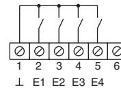
Binary inputs E1...E4: Connect window contact, make or break pushbutton to the terminal strip between terminals 1 and 2...5.
