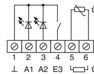
Binary outputs A1, A2: Connect LED or electronic relay to terminal strip between terminals 1 and 2...3. Connect remote sensor between terminals 5 and 6.
