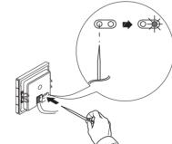
2 Load the physical address and application from the ETS into the push-button: The red programming LED goes out.
