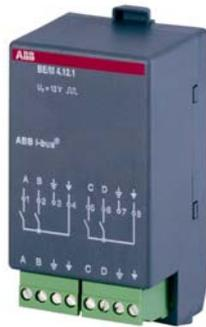
The 4-fold Binary Input Module is operated in any module slot of the Room Controller Base Unit. It has four inputs for reading out floating contacts such as conventional switches and push buttons. The device makes the pulsed scanning voltage (12 V) available.
