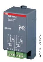
The 2-fold Electronic Switch Actuator Module is snapped into any module slot of the Room Controller Basis Device. Using two semiconductor outputs, it switches two resistive loads such as electrothermal valve drives for heating control. The outputs are noisefree and wear-resistant. The nominal switching voltage is 115 or 230 V.
