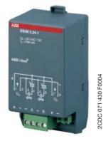
The 2-fold Electronic Switch Actuator Module is snapped into any module slot of the Room Controller Basis Device. Using two semiconductor outputs, it switches two resistive loads such as electrothermal valve drives for heating control. The outputs are noisefree and wear-resistant. The nominal switching voltage is 12 V or 24 V. The internal voltage is supplied via the Room Controller Basis Device. Contact is automatically established when the modules are snapped in place.
