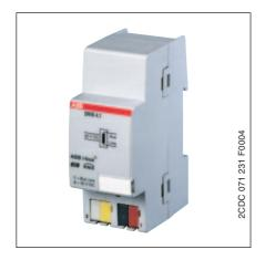
The choke decouples the bus line from the power supply. It can be used together with the power supply unit SV/S 30.640.5 to supply a second EIB line.
