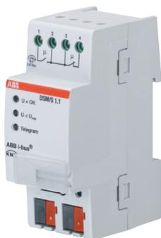
The diagnosis and protection module enables quick diagnostics of the bus state and indicates telegram traffic via an LED. A bus failure ( $U < U_{\min}$ ) can be signalled via the changeover contact. The DSM incorporates a suppressor diode which suppresses transient overvoltages and interference voltage spikes on the KNX.
